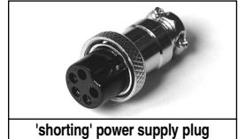
**⚠ Before placing the amplifier onto its chosen place, insert the 'shorting' power supply plug into the PSU socket (7) — see rear panel. Alternatively, you can use the Obelisk X-2 optional auxiliary power supply via this socket (see below 'Upgrade Options'). If this socket is vacant, the amplifier is completely muted because the power amp section is disconnected from the onboard power supply, and thus giving way to connecting the Obelisk X-2.**
